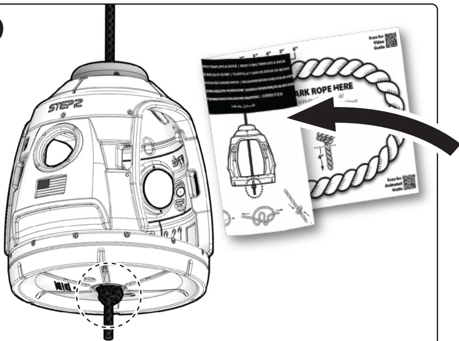
Remove Knot Tying Template & Guide (Next page KT1-KT4) from this instruction sheet. Use Scale template to mark rope to ensure correct rope knot with a minimum 4" tail.
