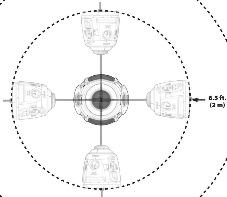
Create an obstruction-free zone with a minimum clearance of 6.5 ft. (2m) from the furthest extent of swing radius.
